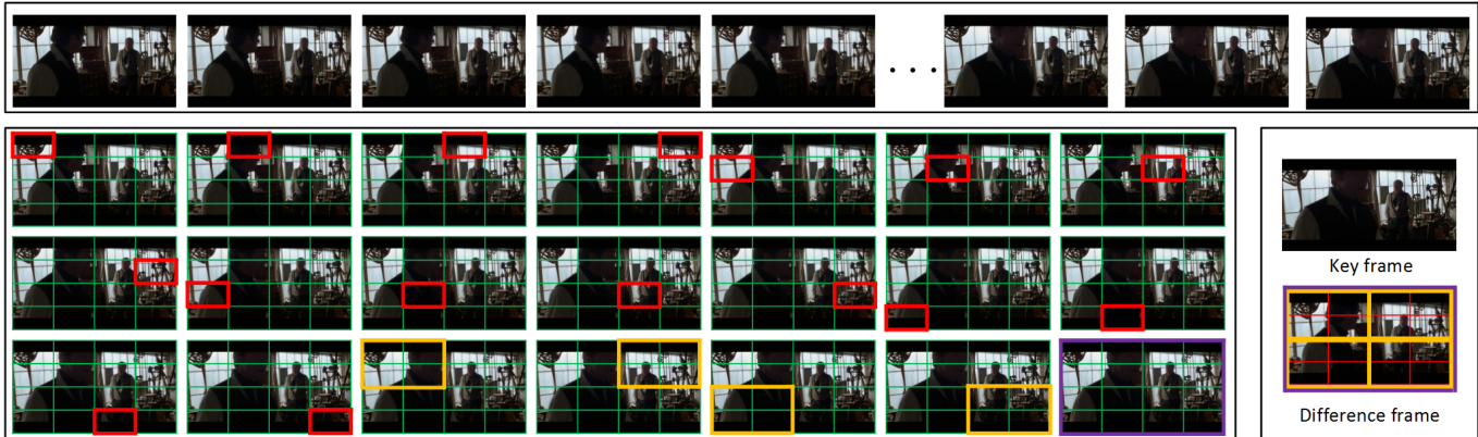
Fig. 2. Illustrations of generating difference frame. All the frames in a shot are shown at the top. We select D pyramid segments from D frames to form difference frame. Each selected segment has the fewest matches to key frame in the same region.
